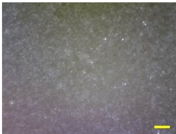
Fig. 1. Micro image of the work surface of a nonstretched rubber band (scale bar is 100 \mu\text{m} ) obtained by means of the optical digital microscope 'Levenhuk' (MODEL D50L NG) [15].
