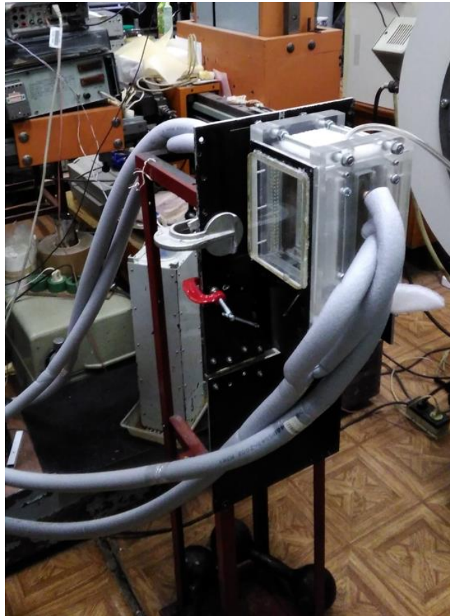
Fig. 2. The rectangular cavity with water. Optical tubes that feed the refrigerant to the heat transfer side plates are visible.
