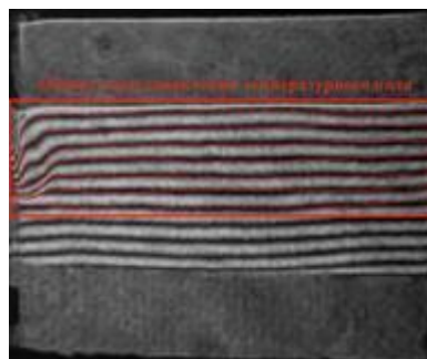
Fig. 5. Approximation by Bezier curves of interference fringes on the shear interferogram.
